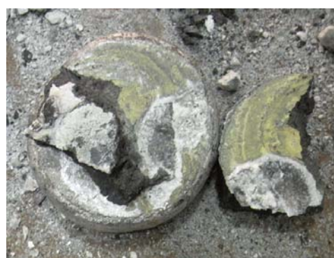
Figure 8. Aluminum block and Al 4 C 3 formation after Test1.
