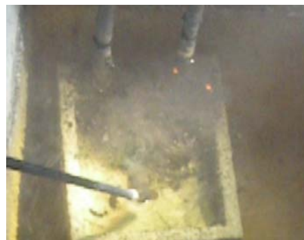
Figure 6. A large amount of black fog and yellow flame appeared after the crust broken.
