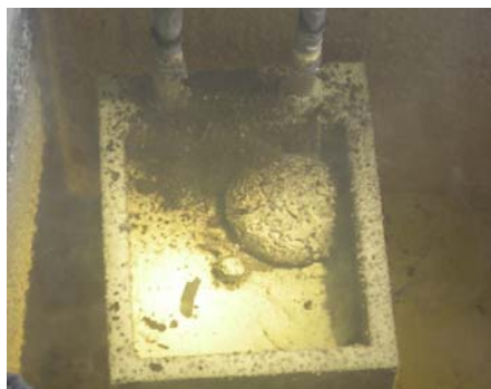
Figure 5. Crust formation after aluminum melts.
